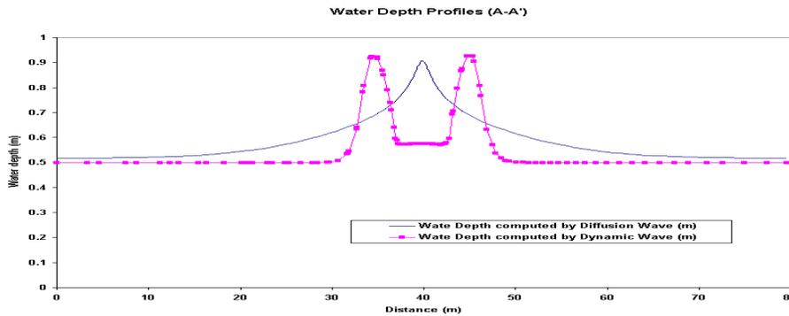
FIGURE 3. Comparison of Computed water depth profile for Example 2.
