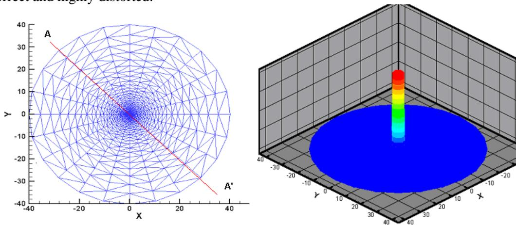
FIGURE 2. Finite element and initial condition for the circular dam problem
