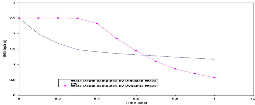
FIGURE 4. Comparison of Computed water depth hydrographs for Example 2.
