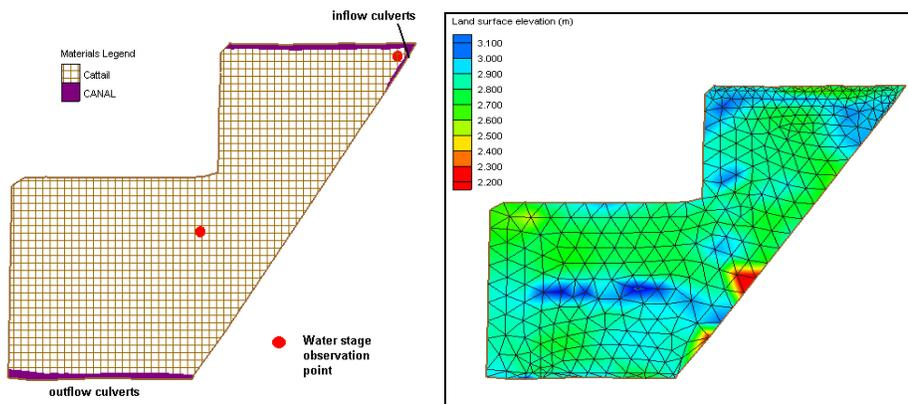
FIGURE 5. Finite element mesh and other model data for Example 3.
