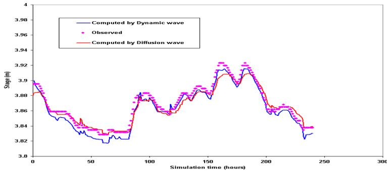
FIGURE 7. Comparison of Observed and Computed Stages for Example 3.
