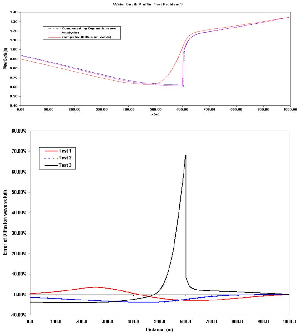
FIGURE 1. Water surface profiles for Test Problem 3 and error of DIW solutions
