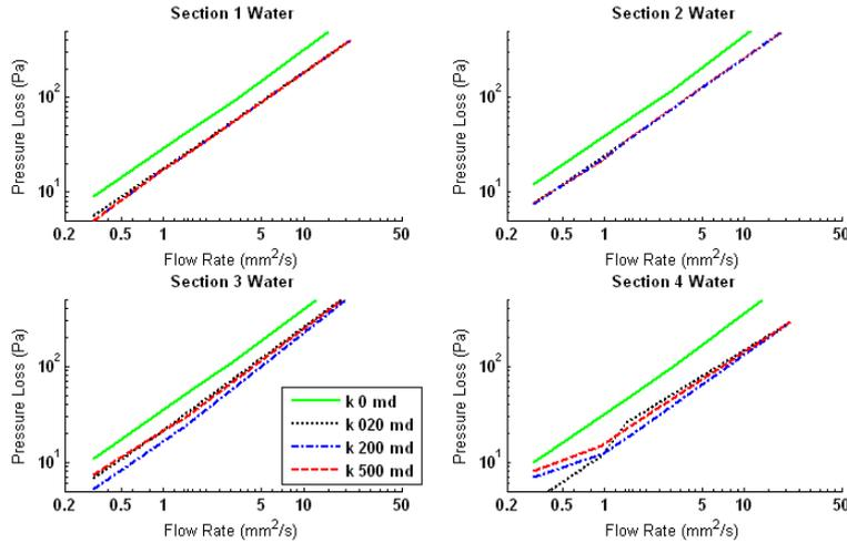
FIGURE 5. Pressure loss calculated for range of flow rates, water.
