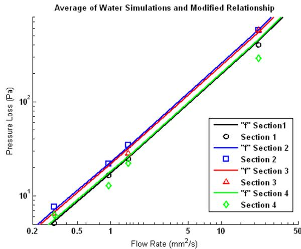
FIGURE 7. Comparison of revised  $f$  relationship and water simulation results.
