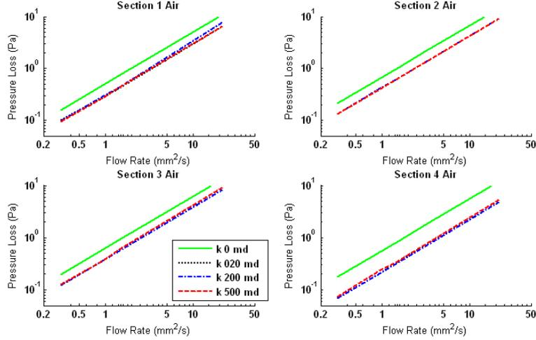
FIGURE 4. Pressure loss calculated for range of flow rates, air.
