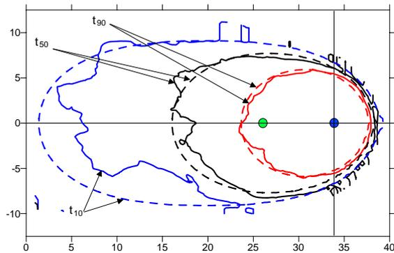
FIGURE 6. Percentiles  $t_{10}$ ,  $t_{50}$  and  $t_{90}$  for 200 hours isochrones in aquifer with  $e = 8$  and  $\sigma_Y^2 = 0.5$ .  $N_{MC} = 1000$ .
