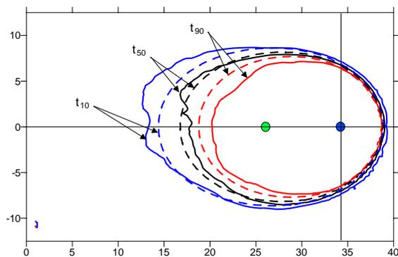
FIGURE 4. Percentiles  $t_{10}$ ,  $t_{50}$  and  $t_{90}$  for 200 hours isochrones in aquifer with  $e = 8$  and  $\sigma_Y^2 = 0.1$ .  $N_{MC} = 200$ .
