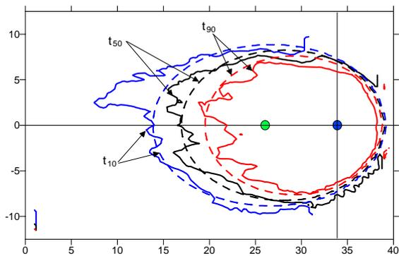
FIGURE 5. Percentiles  $t_{10}$ ,  $t_{50}$  and  $t_{90}$  for 200 hours isochrones in aquifer with  $e = 1$  and  $\sigma_Y^2 = 0.5$ .  $N_{MC} = 1000$ .
