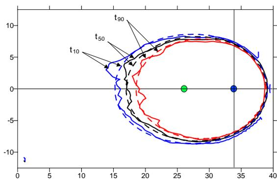
FIGURE 3. Percentiles  $t_{10}$ ,  $t_{50}$  and  $t_{90}$  for 200 hours isochrones in aquifer with  $e = 1$  and  $\sigma_Y^2 = 0.1$ .  $N_{MC} = 200$ .
