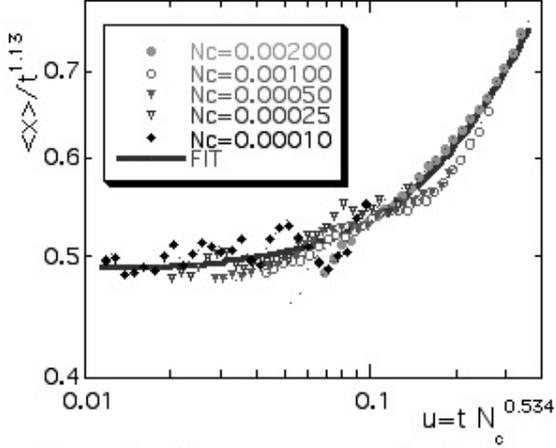
Figure 1 The crossover regime between fractal capillary fingering (small  $u$ ) and fractal viscous fingering (large  $u$ ) is shown for viscosity ratio,  $M = 10^4$ , and five capillary numbers.
