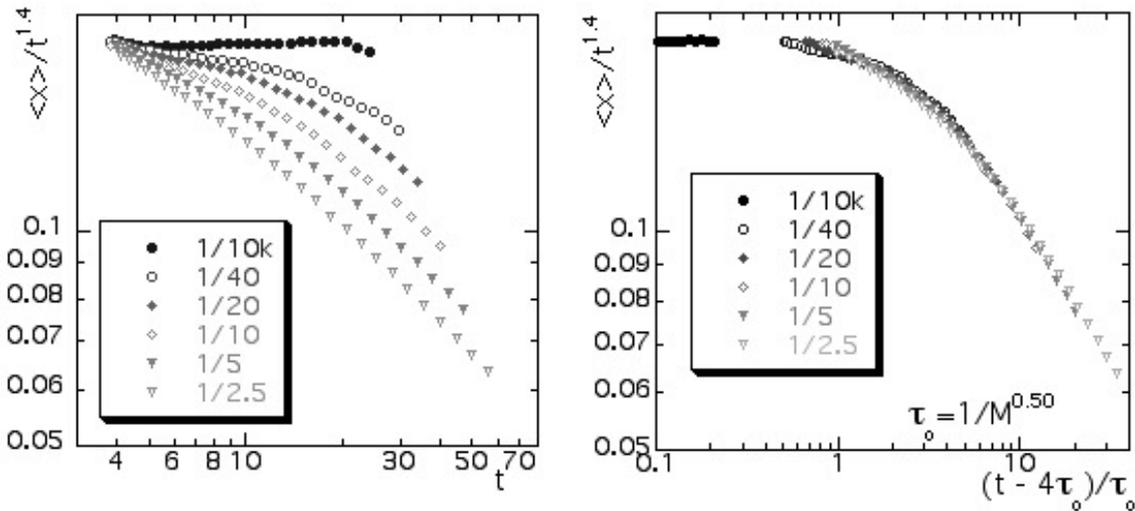
Figures 8.a(left) and 8.b(right) The data for the average position of the injected fluid are presented for capillary number  $N_c=0.1000$  and for viscosity ratios from  $M=0.0001$  to  $M=0.4$ .
