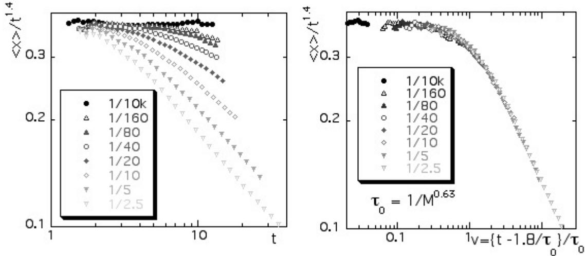
Figures 6.a(left) and 6.b(right) The data for the average position of the injected fluid are presented for capillary number  $N_c=0.0040$  and for viscosity ratios from  $M=0.0001$  to  $M=0.4$ .
