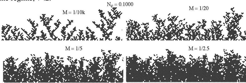
Figure 7 Breakthrough patterns of injected fluid for one of ten realizations for capillary number  $N_c=0.1000$  and for viscosity ratios from  $M=0.0001$  to  $M=0.4$ .
