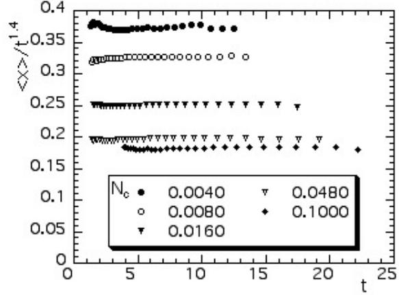
Figure 2 shows the fractal viscous fingering behavior,  $\langle x \rangle = B t^{1.4}$  for viscosity ratio,  $M = 10^4$ , and for five large capillary numbers. The smallest times are omitted in this figure.
