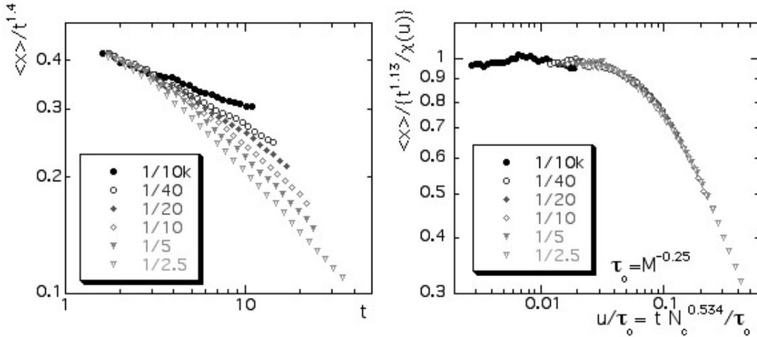
Figures 4.a(left) and 4.b(right) The data for the average position of the injected fluid are shown for the capillary number  $N_c=0.0005$  and for viscosity ratios from  $M=0.0001$  to  $M=0.4$ .
