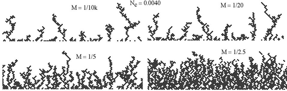
Figure 5 Breakthrough patterns of injected fluid for one of ten realizations for capillary number  $N_c=0.0040$  and for viscosity ratios from  $M=0.0001$  to  $M=0.4$ .
