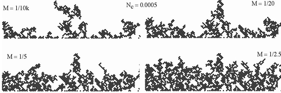
Figure 3 Breakthrough patterns of injected fluid for one of ten realizations for capillary number  $N_c=0.0005$  and for viscosity ratios from  $M=0.0001$  to  $M=0.4$ .
