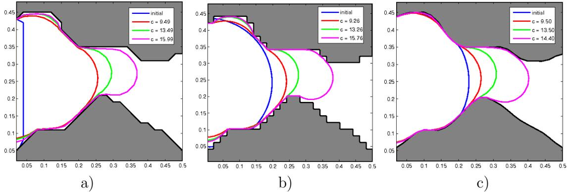
FIGURE 4. Simulation in a 2D throat cut out from a slice of a segmented 3D X-ray microtomography image. Critical curvature zero level set in each plot is shown in magenta. a) Simulation with a crude mask directly from a segmented image. b) Simulation with a crude mask from the segmented image magnified 5 times (each voxel replaced by  $5 \times 5$  voxels of the same value). c) Mask obtained from the segmented image as for a), but reinitialized before the simulation.
