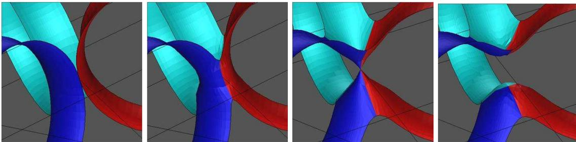
FIGURE 2. Surface Evolver simulation [Noble and Bryant, 2002] of constant curvature surfaces at decreasing values of curvature. Initial configuration (left) consists of pendular rings (in different colors) around 3 neighboring spheres (spheres not shown). With curvature gradually decreasing, wetting phase rings touch, merge, and coalesce. This sequence of events corresponds to “snap-off” of the nonwetting phase that previously occupied the pore throat between the three spheres.
