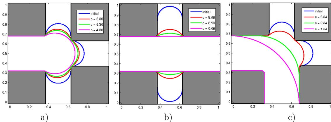
FIGURE 5. Imbibition in square pores with variable combinations of attached throat channel widths. Only a few steps are shown in each figure for clarity, with the final stable stage outlined in magenta color. a) Imbibition starts from drainage curve with 3 menisci. b) Imbibition starts from drainage curve with 2 “opposite” menisci. c) Imbibition starts from drainage curve with 2 “neighboring” menisci.
