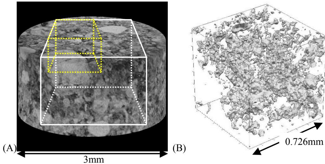
FIGURE 2. (A) A larger grey scale image and (B) a smaller binalized image of the microtomography of the sample. The image (A) has a macro-porosity of 0.106 identified by micro-CT with a resolution of  $5.67\mu\text{m}/\text{voxel}$  and the binalized image (B) extracted from the image (A) has a porosity of 0.104.
