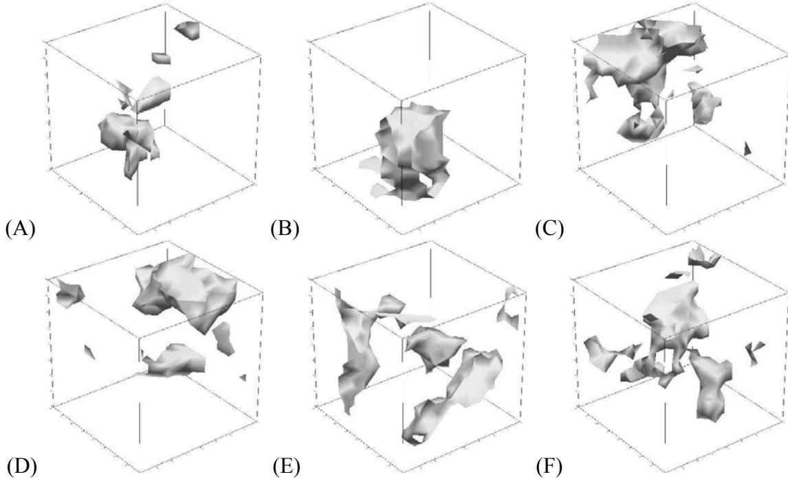
FIGURE 4. Extracted subsets (size= $128^3$ ) from the 3D microtomography of macro-pores with different porosity values. (A)  $\phi=0.05$ , (B)  $\phi=0.075$ , (C)-(F) have almost same macro-porosity,  $\phi=0.10$ , but the locations of these subsets taken in the measured microtomography are different.
