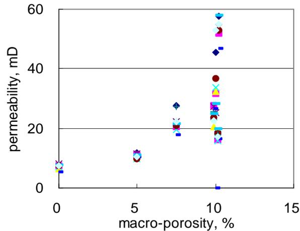
FIGURE 5. Variation of computed permeabilities in combined images with different macro-porosities. As the macro-porosity is increased, the range of permeabilities becomes large for these small reconstructed images due to heterogeneous distributions of macro-pores. The range of permeability will be reduced as the size of the image is increased.
