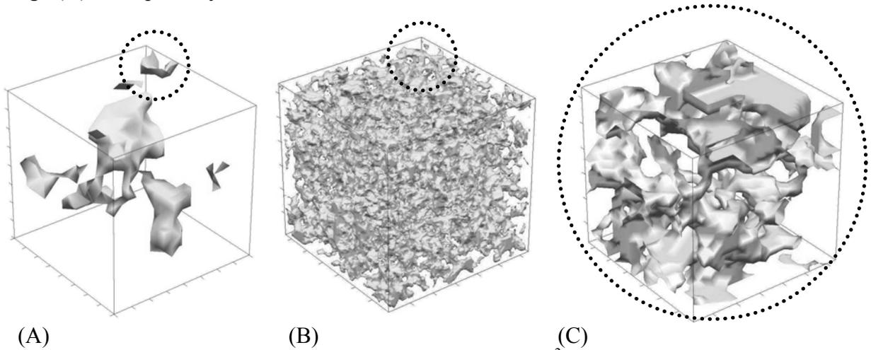
FIGURE 3. Smaller parts of reconstructed images (size= $128^3$ ,  $0.709\mu\text{m}/\text{voxel}$ ). (A) A part of the microtomography image with macro-pores that are not well connected (porosity,  $\phi = 0.0991$ ), (B) one realization of a reconstructed image using MPS ( $\phi = 0.221$ ) and (C) a smaller combined image of (A) and (B) with the subset of the volume marked by the dotted circle (size= $32^3$ ,  $\phi = 0.299$ ).
