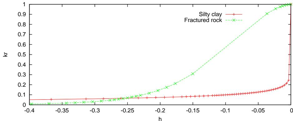
FIGURE 1. Relative hydraulic conductivity for silty clay and fractured rock
