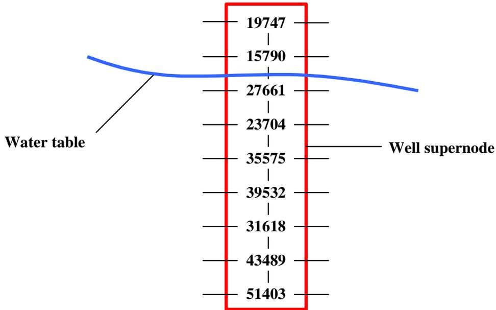
FIGURE 6. Modeling a well with a well supernode
