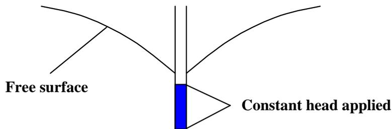
FIGURE 5. Partially penetrating well with free surface or water table
