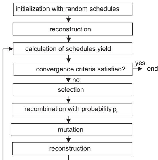
FIGURE 4.1. Flowchart of the algorithm for the optimization of irrigation schedules.
