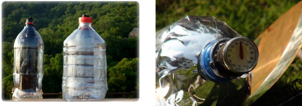
**Figure 4.** Solar-thermal water heater designs (left) system testing (right)
