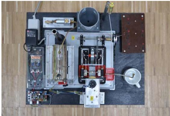
**Figure 1a** A bird's view of the steam engine part of the electric energy system including the transformer, but without power electronics.
