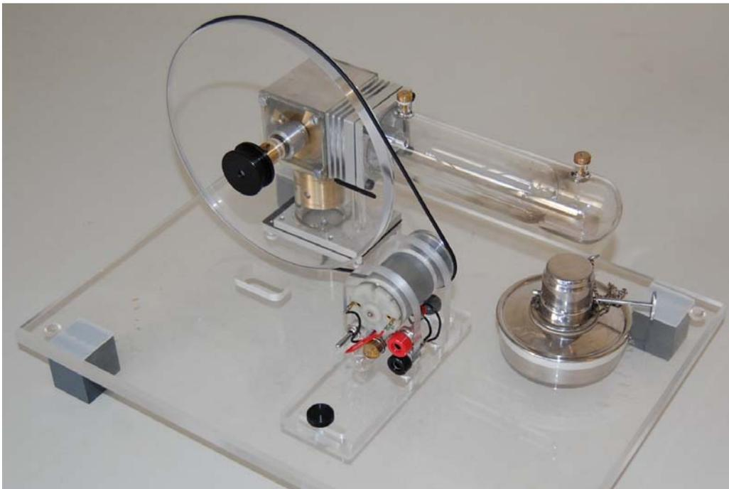
Figure 3. Transparent Stirling engine used for second assignment
