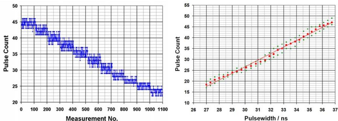
Figure 6. TDC-counts as a function of reflector displacement (left) and calibration
